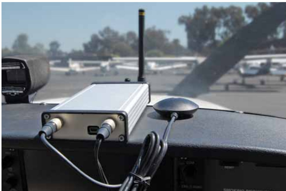
SkyRadar's $1,200 ADS-B receiver includes a plug-in, WAAS-capable GPS receiver to get an accurate aircraft altitude to aid in displaying vertical distance from terrain and traffic.
