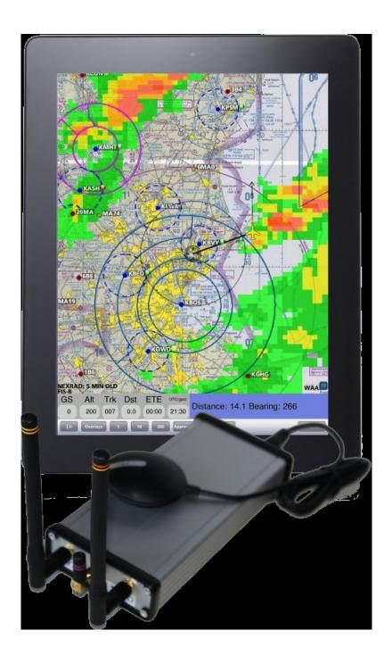
Today, ADS-B ground stations broadcast weather all the time for free. **SkyRadar** receives this signal, decodes it and displays color coded weather data—METARs, TAFs, NEXRAD, Winds Aloft, PIREPs, NOTAMs—as an overlay on its moving map. This enables the pilot to adjust the flying route accordingly, thus dramatically increasing flight safety while reducing fuel costs.
