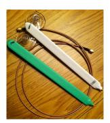
Set of Remote Antennas (978MHz+1090MHz) for the Dual Band receiver {{antennaSet}}
